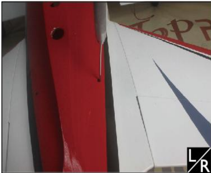
44. Lock the stabilizers to the fuselage by screws from the top of the tail fuselage.
