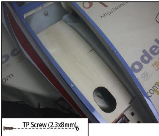
37. Put the plywood plate in the fuselage.
