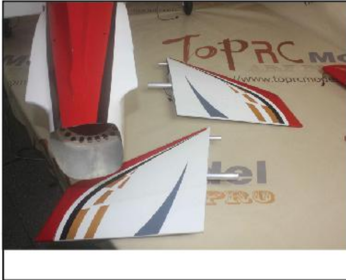
44. Lock the stabilizers to the fuselage by screws from the top of the tail fuselage.
