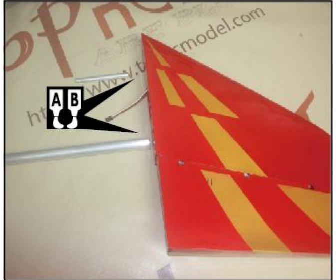
45. Glue the vertical tubes to the vertical fin.
