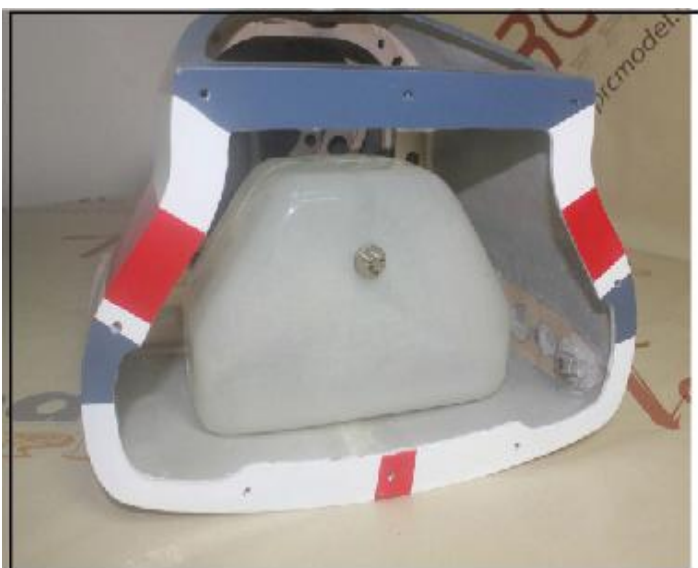
34. Put the fuel tank into the fuselage.
