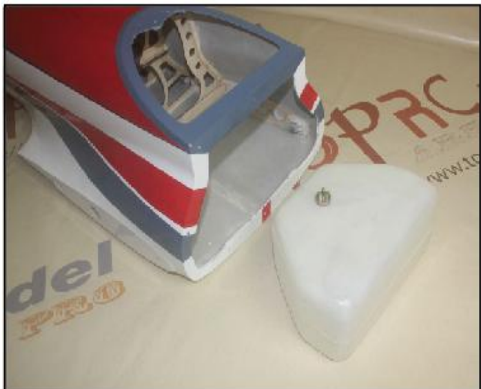
34. Put the fuel tank into the fuselage.
