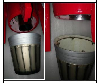
19. Fix the tail pipe through assembly the 3mm ply tail pipe frame, see pictures below .
