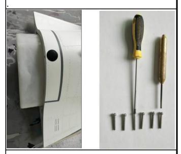
29.Assemble the fuselages together tightly.
