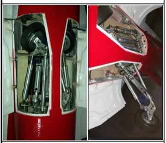
26. Make sure the gears can be completely retracted during work .
