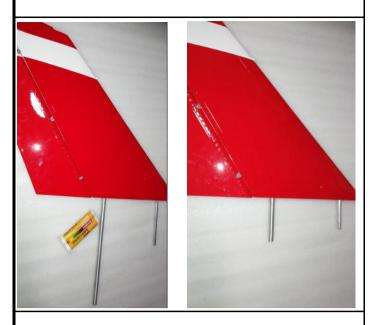
12. Assemble the vertical fin to the tail fulse .
