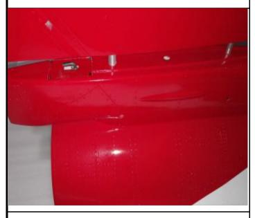
13. Lock the vertical fin by screws from the tail fuselage holes, make sure the rudder can move smoothly .
