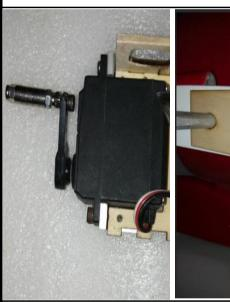
7. Assemble the stab servo to appropriate position in the fuselage with screws and make sure the screw with bearings can move through the slot smoothly.
