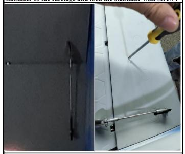
14.Assemble the rudder arm wire to the tail fuselage as illustration.
