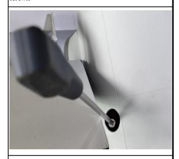
12. Assemble the servo to appropriate position in the stabilizer, and connect the horn in the elevator .
