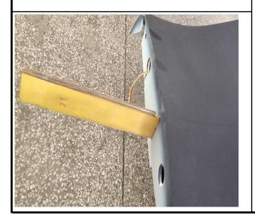
10. Assemble the out wing to the center wing and lock them with screws.
