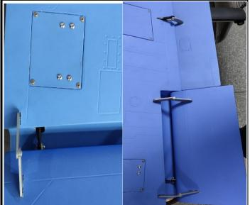
4. Assemble the flap on the center wing, put the flaps together, trim slots to appropriate position in center wing trailing edge and flap, apply instand type ABglue to the slots in the flap and horns. Connect the servo to the horn with screws.
