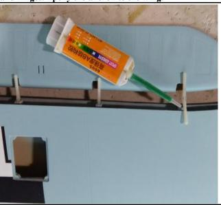
4. Epoxy the aileron to the wing, Keep some space between the trailing edge and the aileron to make sure it can rotate smoothly.
