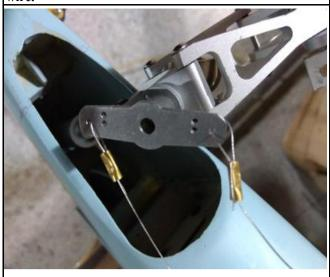
20. Drill a small hole to appropriate possition in the fuselage, connect the rudder to the servo in the fuselage via steel wire.
