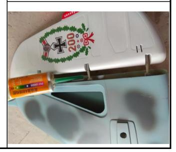
16.Picture of the rudder install ready, make sure it can rotate smoothly.
