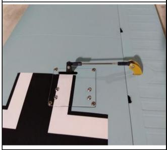
10. Connect the fiber horns in the flap to the servo arms with the linkage and lock each side with screws and nut.
