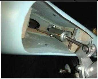
18. Fix the air cylinder to the tail fuselage.
