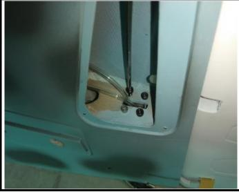
19. Connect the arm of the tail landing gear with steel wire.
