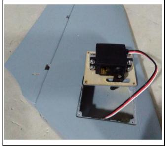
16.Fix the servo trays to the stab with screws, Connect the fiber horns to the servo arms with the linkage and lock each side with screws and locknuts.
