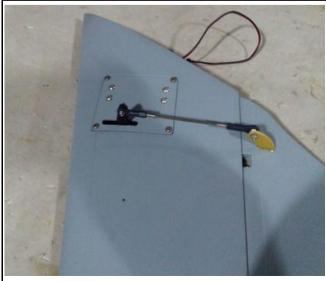
17.Assemble the servo tray with servo assembled to the tail fin.
