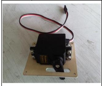
15. Assemble the servos to the stab servo trays.
