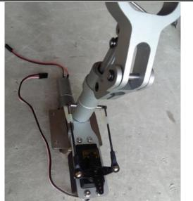
29.Assemble the nose retract to the fuselage with screws and assemble the back half nose gear door.
