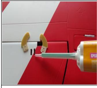
5. Apply AB glue to the slots in the flaps and assemble the horns into them.
