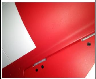
22.Assemble the inner gear door to the fuselage with screws
