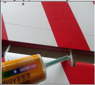
4. Apply AB glue to the slots in the ailerons, and assemble the horns into them.
