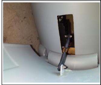
Accessory list for the installation of main gear door. Pin hinge Pin hinge Plastic Horn (2mm) 2 Screw (2x8mm) 16 Push rod (28x2mm) 2 Clevis (2mm) 4 Screw (2x12mm) 4 OLocknut (2mm) 4 21.Trim slots in the gear door,glue the pin hinges into the gear door and fuselage, assemble the gear door to the fuselage with screws.
