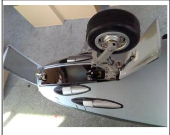
**30.Connect the back half nose gear door to the landing gear with push rood and screws.**
