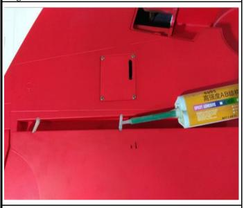
2. Epoxy the flap to the wing, Keep some space about 1mm width between the trailing edge and the flap.
