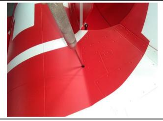
42.Assemble the stab to the fuselage through the stab tubes and lock them with screws.
