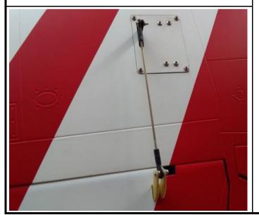
9. Fix the servo trays with servo assembled to the wings with screws.
