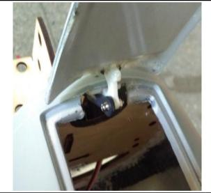
28. Assemble the nose landing gear and the servo to the nose retract.
