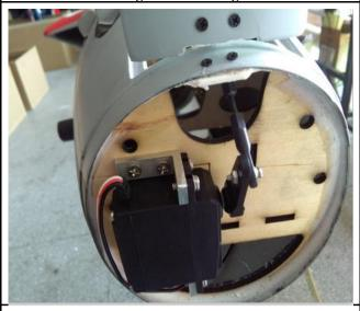
27. Connect plastic horn to the servo via push rod and screws.
