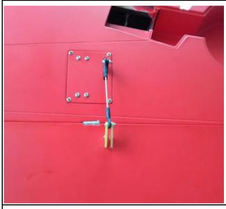
11.Put the plastic screw in the holes of wing, fasten the bomb socket with bombs to the wing.
