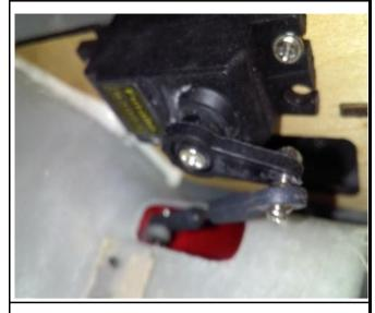
25.Connect the innner gear doors and the servos througn the slot in the fuselage
