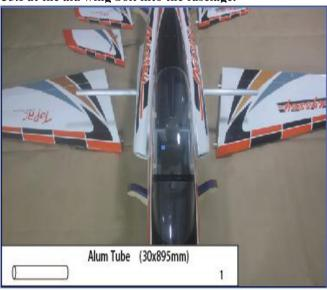
36.Assemble the wing to the fuselage through the wing bolt.
