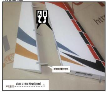
15.Assemble the rudder to the vertical fin and make sure it can move freely.
