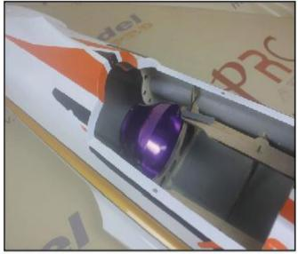
**30.** Assemble the Turbine and tail pipe.
