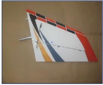
41.Put the vertical fin to the fuselage.
