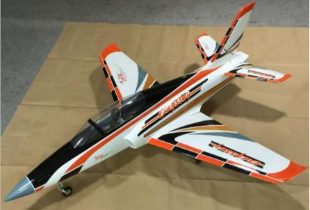
Specification: Wing Span: 2320mm/91in Length: 2190mm/86in Flying Weight: ~12kg Turbine: 10~14kg Radio: Min. 9 ~ 11 Servos required R/C System: 8+ channel radio system C.G: 210~215mm from the leading edge
