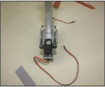
23.Assemble the steering linkages.
