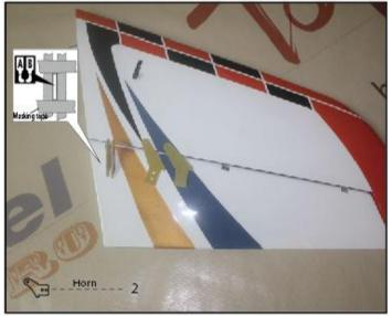
18.Measure the deepth to confirm what the servo position will be and open a small slot for the servo arm.
