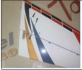
**20.**Connect the fiber horns to the servo arms with the linkage and locked each side with screws.
