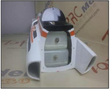
28.Put the tail pipe to the fuselage.
