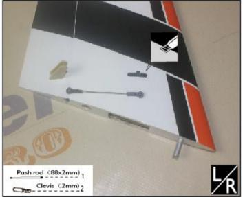
13.Connect the fiber horns to the servo arms with the linkage and locked each side with screws and locked nut.
