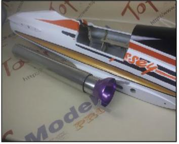
**29.**Fix the tail pipe to the fuselage with screws.
