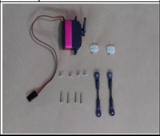
45.Assemble the nylon horn to the air brake inner side, assemble the air brake servo to appropriate position in the fuselage, connect the horn to the servo arm with push rod.
