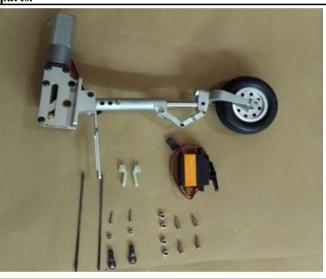
38.Assemble the nose servo to the nose gear.
