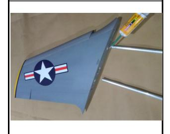
65.Fix the wing tube to the holes tightly.
