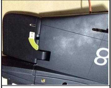
**30.Put masking tape around the slot to keep the plane body clean after work done.**
