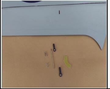
9. Before glue the arm to the slot, put masking tape around the slot to keep clean.
