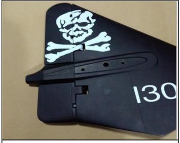
24.Measure the deepth of the rudder servo position.
