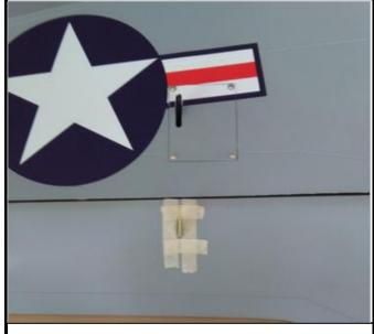
11.Connect the arm of the flap and servo arm with push rod.
